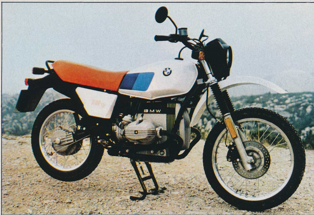
Below: Sump on all the 1981 models is deeper, the R80G/S using a bash plate.
