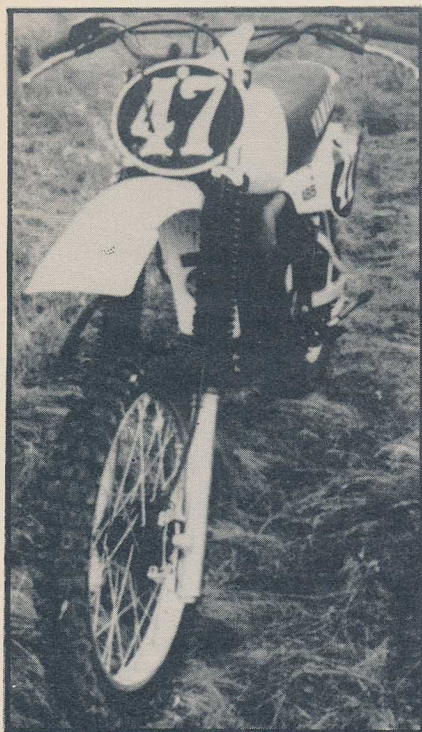
Front forks are air assisted.
