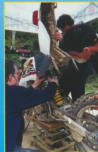
After fitting, each shock was set up for the test rider and adjusted after a few practice laps. Above left: Air Xo shock could be used with or without the Honda linkage
