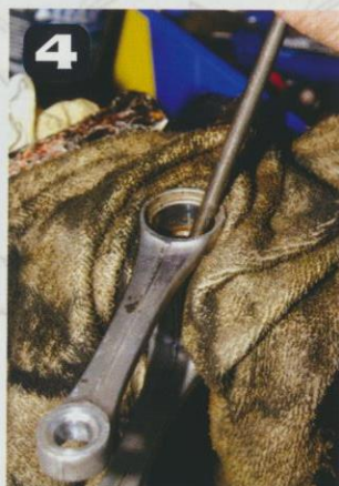
Make drifting the old bearings out a bit easier by securing the linkage in a vice
