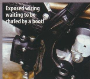
Speedo sensor looks vulnerable and reads off the rear wheel...
