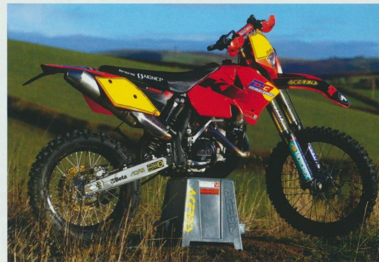
David's E3 winning bike is all about smooth usable power. GMX oversize rads help keep the 56hp lump nice and cool. Besides the numerous engine mods, the biggest difference over a standard 525 is the use of factory WP suspension...
