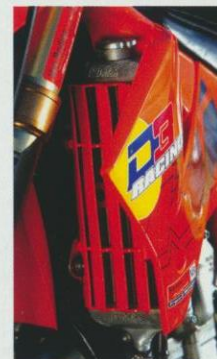
David's E3 winning bike is all about smooth usable power. GMX oversize rads help keep the 56hp lump nice and cool. Besides the numerous engine mods, the biggest difference over a standard 525 is the use of factory WP suspension...
