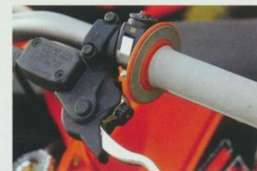
Above: A competition kit now comes 'free' with every EXC model Left: Black painted frame contrasts with the orange spring Right: Two-stroke models get a Brembo hydraulic clutch for smoother operation
