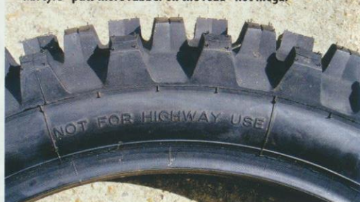
MX tyre - puts more rubber on the road - not illegal
