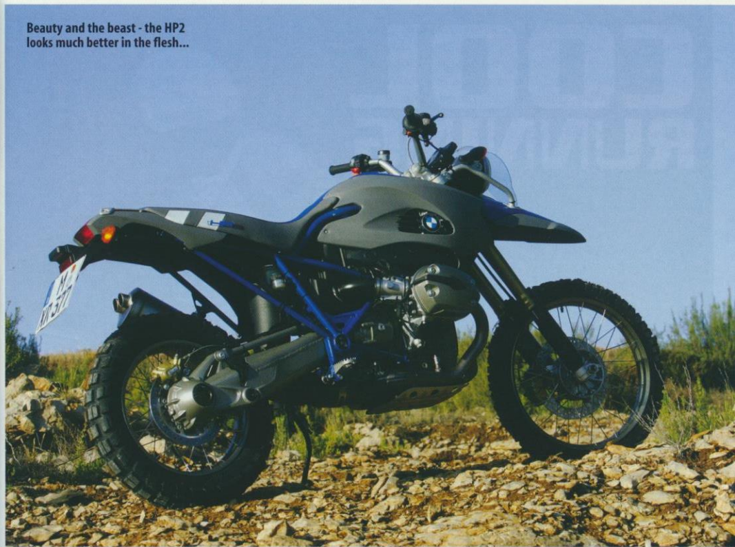
Left: A breath of fresh air - BMW are the first to put an air-shock on a production bike... Smoothly does it - the 105bhp slightly modified Boxer engine powers the HP2...
