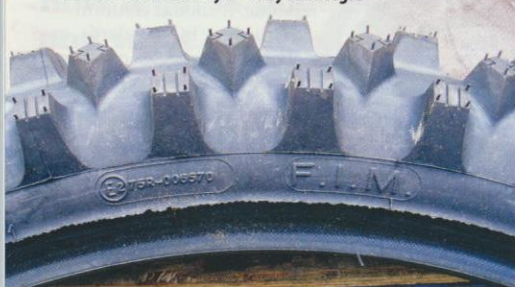
E-marked FIM enduro tyre - fully road legal
