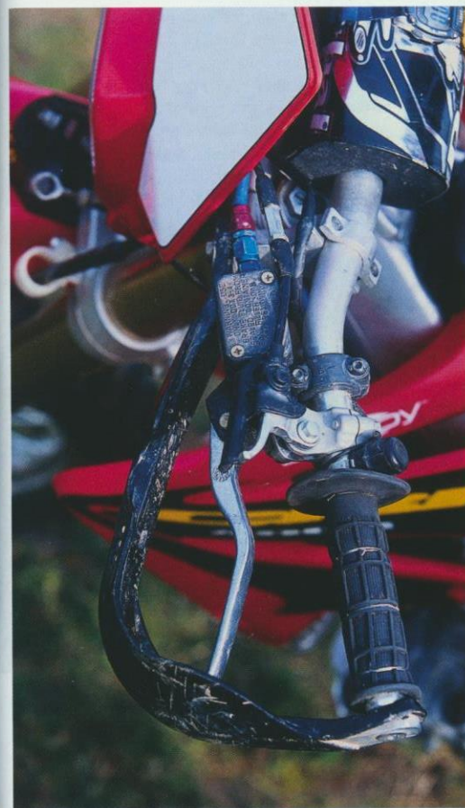
Main pic: The left bar has what looks like a hydraulic clutch lever, but is in fact a rear brake (plus the CRF's hot-start lever... Above: Clutch cable to the actuating arm is replaced by one of three different weight springs which alter the amount of clutch slip and the speed of the take up. New versions of the clutch do away with this external spring. Right: Mark's happy!
