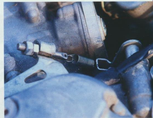
Main pic: The left bar has what looks like a hydraulic clutch lever, but is in fact a rear brake (plus the CRF's hot-start lever... Above: Clutch cable to the actuating arm is replaced by one of three different weight springs which alter the amount of clutch slip and the speed of the take up. New versions of the clutch do away with this external spring. Right: Mark's happy!
