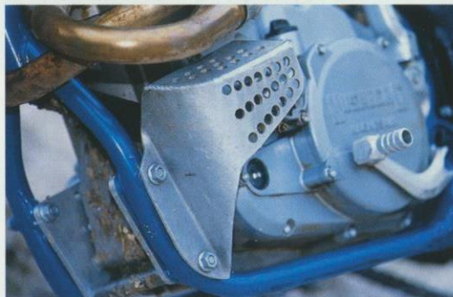
Right: Drilled alloy water-pump cover is a non-standard item
