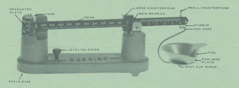
The Redding Model No. 2 Powder and Bullet Scale is one of the most accurate and sensitive scales available. It features a simple two counterpoise system and magnetic dampened beam for fast and accurate measurements. A graduated over and under plate provides additional speed and ease of operation, allowing the operator to check variations in powder charges or bullet weights without adjusting the counterpoises.
