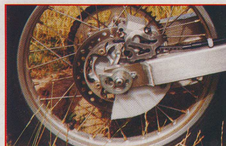
Rear disc is ok – but no more than that. Note snail-cam adjusters ... very useful on the trail
