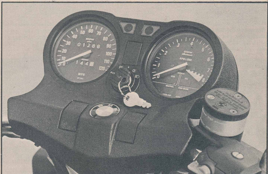
The red line starts at 7500rpm and the engine will happily rev past 8000. Maximum power is quoted at 7250rpm.
