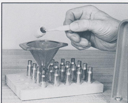
AUTO PRIME is hand held and requires special, but inexpensive shell holders. Safe only with CCI or Winchester brand primers.
