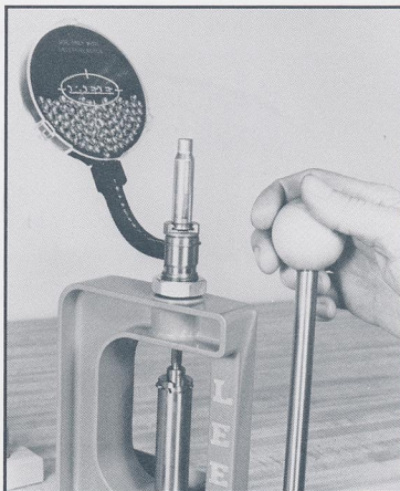
AUTO PRIME II fits in your press and uses the same shell holder used for reloading. Safe only with CCI or Winchester primers.
