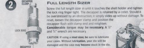
Carbide Sizing Dies **Need No** Lubrication
