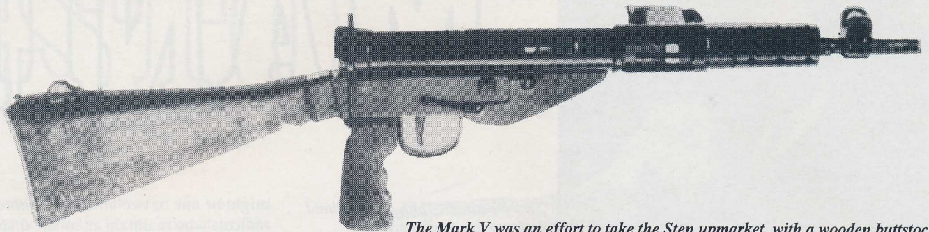
The Mark V was an effort to take the Sten upmarket, with a wooden buttstock and pistol grip, No. 4 foresight and bayonet lugs, and generally more careful fit and finish throughout. The troops could scarcely have failed to notice how much cruder and less satisfactory the earlier Stens were than the MP40's and Berettas on the other side.
