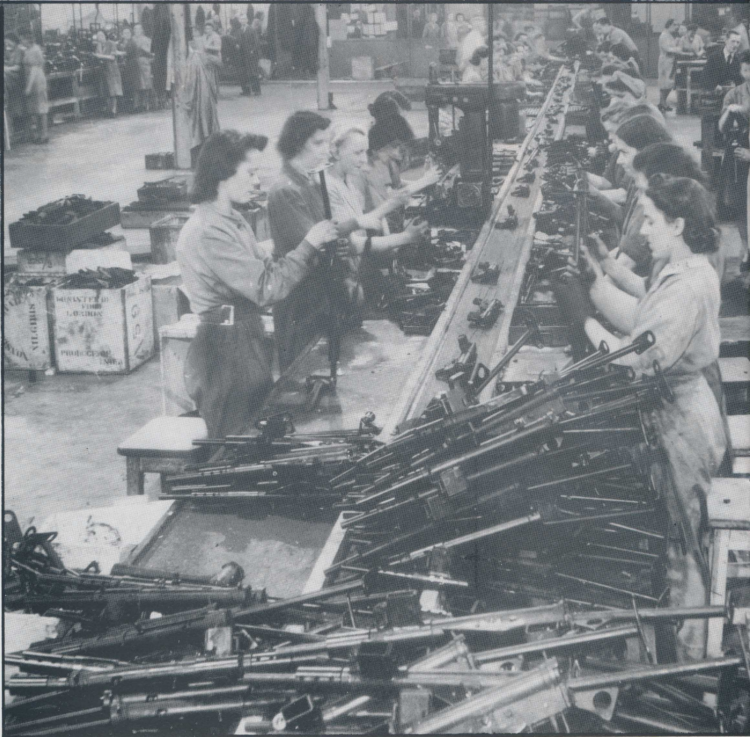
The Sten was made for the most part by women, many of whom lived in Ministry of Supply hostels near the works. A surprising number were refugees: Belgian, Polish, German, Hungarian, Czech, Austrian, even Greek names abound. Shown here is the final assembly line with a stack of finished Mk. II's in the foreground. Work was fed onto the line from the fitting benches to the right and the manufacturing area to the left, with assembly's progressing as the receivers moved up the central conveyor. The two ladies nearest the camera are fitting the stocks on.
