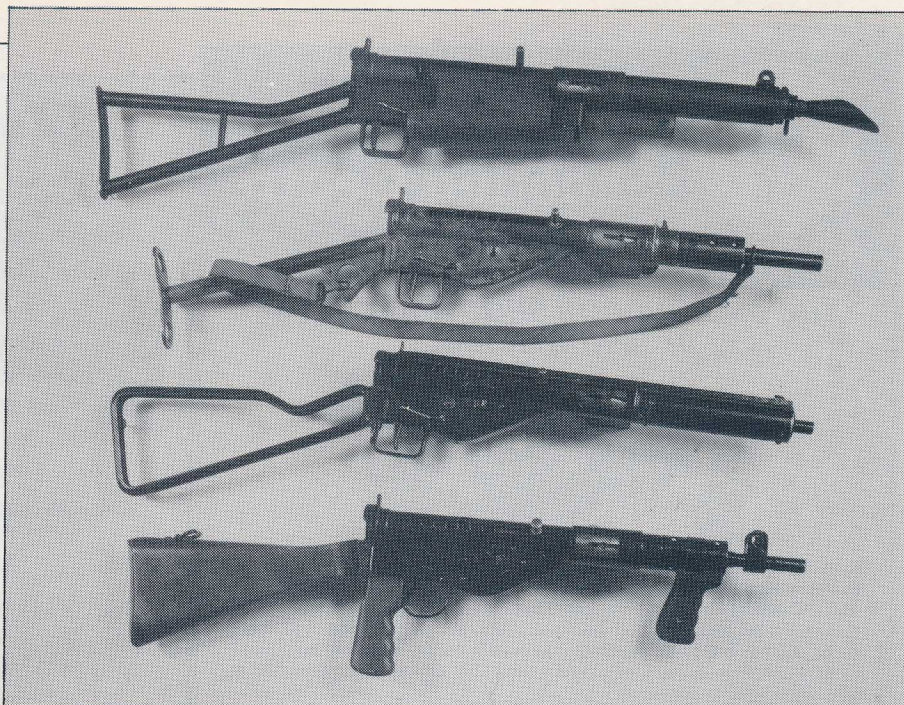
From top: Stens Mark I, II, III and V. Mark IV was not produced. There was also a Mark I* that deleted the flash hider, wooden fore-end and folding forward pistol grip. The Mark III used a stamped rather than a tubular receiver, and was spot welded along the sighting rib where the tabs at either end of the blanking met.
