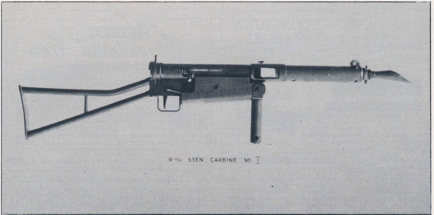
The Mark I Sten was a desperation measure, designed in two months to enable an unarmed people and a disarmed army to meet an anticipated invasion. Note the flash hider cum muzzle brake and the wooden fore-end, deleted on later models, as was the folding forward grip, which made rather a neat monopod. The bolt handle, which made safe by turning up on later models, turns down on the Mark I. Nor did barrels interchange with later Marks.
