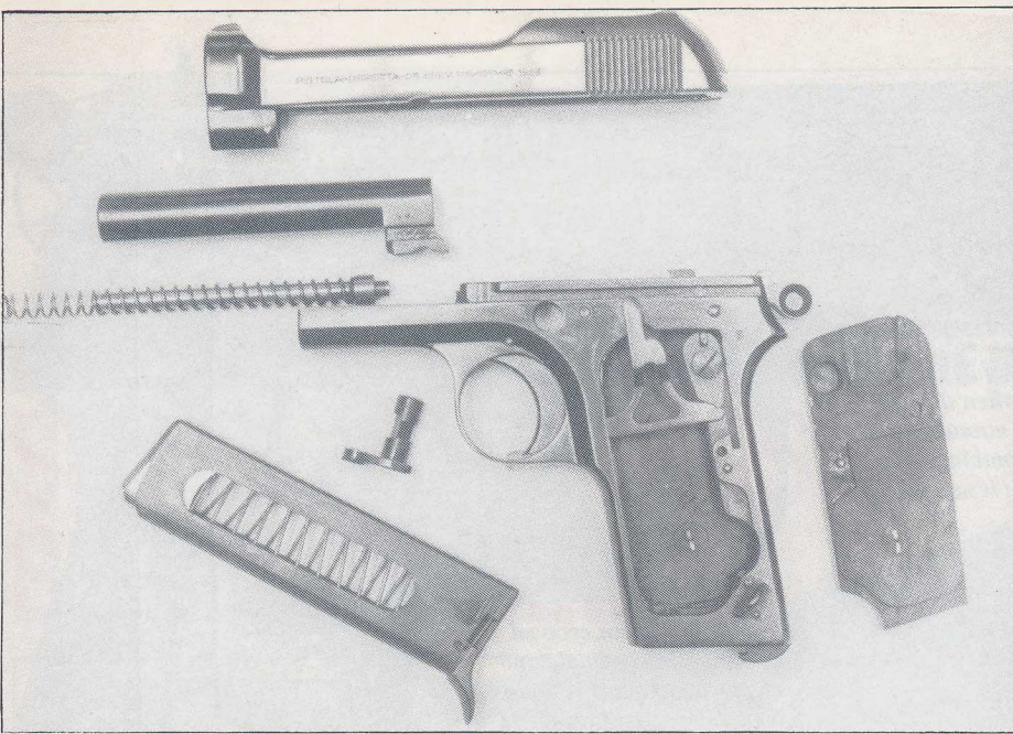
Further significant changes on the 1923 Model (above) were the incorporation of the disconnecter as a vertical extension of the trigger bar, and a more rigid arrangement for mounting the barrel into the frame. Rails on the barrel lug engaged corresponding rails in the frame forward of the magazine well.
