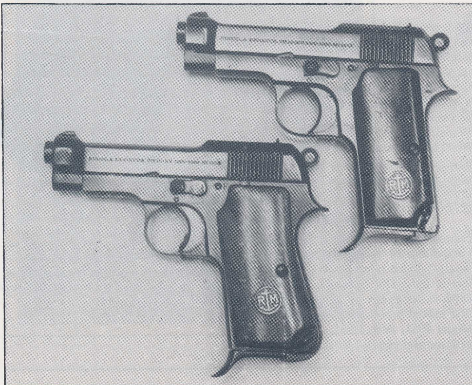
As these two examples show, Marengoni was continuing to sculpt his pistols toward an aesthetic that the 1934 Model was to exemplify. This pair is in .32 ACP and, as the "Regia Marina" escutcheon indicates, saw service with the Italian Navy. The upper gun is the 1931 Model, while the one beneath it, with the more comfortable and pointable angled backstrap, is the 1932 Model and apparently identical to the formally adopted Model of 1935.
