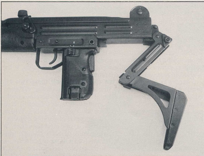
The folding stock part closed. The stock is locked in the short position by means of the lug seen under the body behind the pistol grip.
