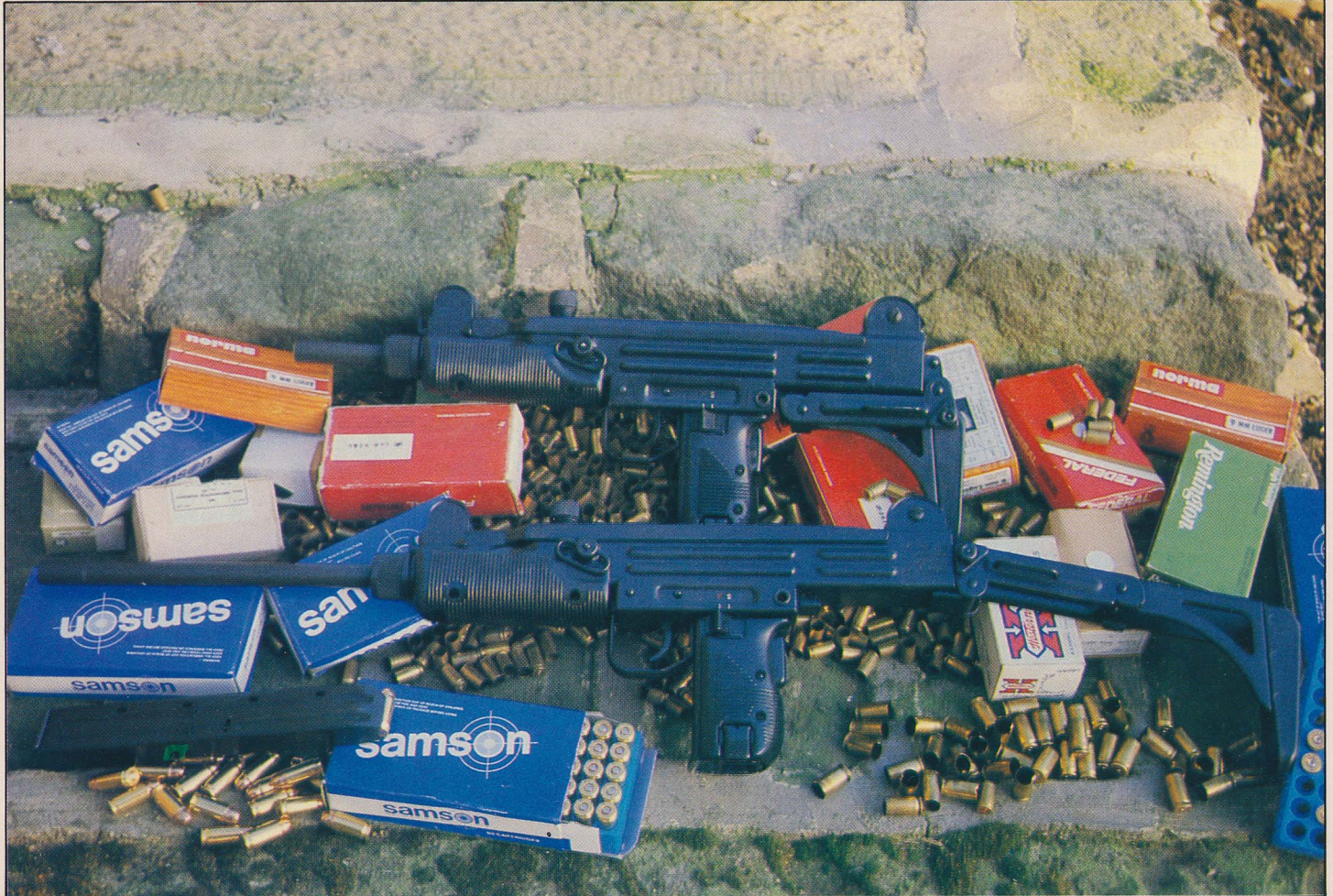
The new .45 Uzi Carbine with 16 inch barrel and stock extended contrasted with the short barrel 9mm carbine with its stock folded.
