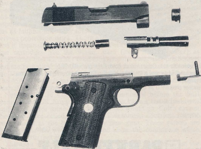
The Officer's ACP field stripped. Note the double recoil spring.
