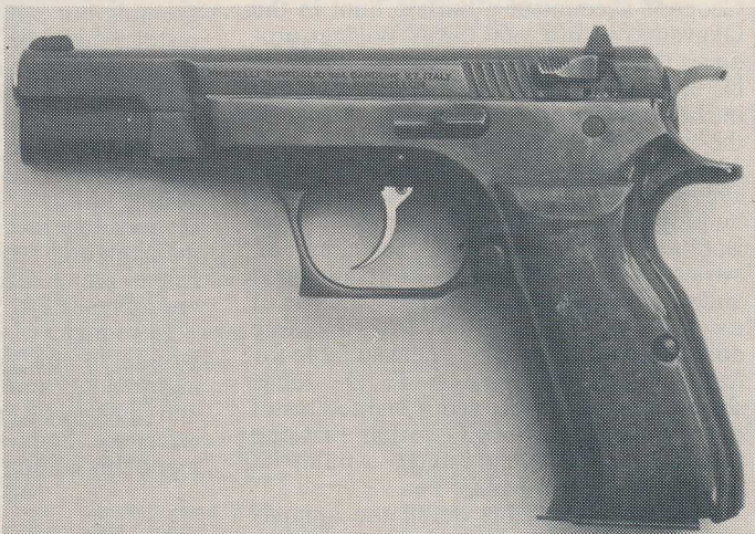
The left side of the pistol. Note the position of the safety, locking pin and magazine release.
