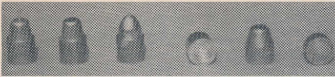
Swaged bullets, two showing metal bleed on nose, others nipped clean. The pointed bullet was for use in a .450" Bulldog revolver.
