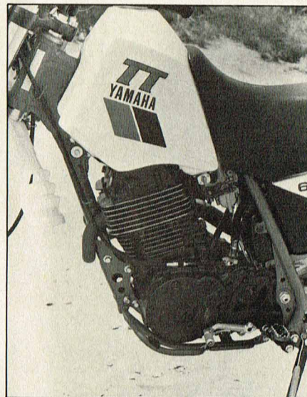
Based on the XT550 engine, the TT600 is a good, strong powerplant from idle to peak revs.
