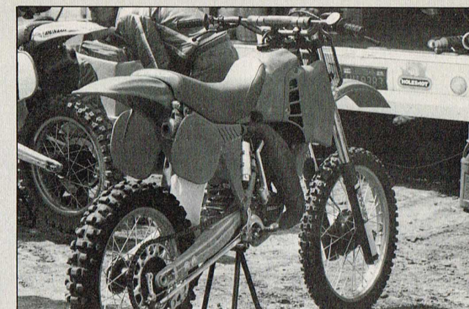
Nearly all of the works bikes use 38mm carbs. This is an easy way to pull more mid-range and some top end out of a 125. Upping your stock carb two millimeters is a good start. Carrying extra gearing to the track should be a must. As you can see, Team Yamaha has wheels with optional-sized sprockets. Most people can't afford this extravagant route. Simply take a smaller countershaft sprocket and a couple of rear sprockets with varying number of teeth.
