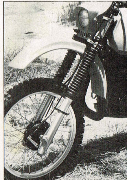
Although the Kawa forks require air, the action is good. The front brake is weak considering the size of the bike.
