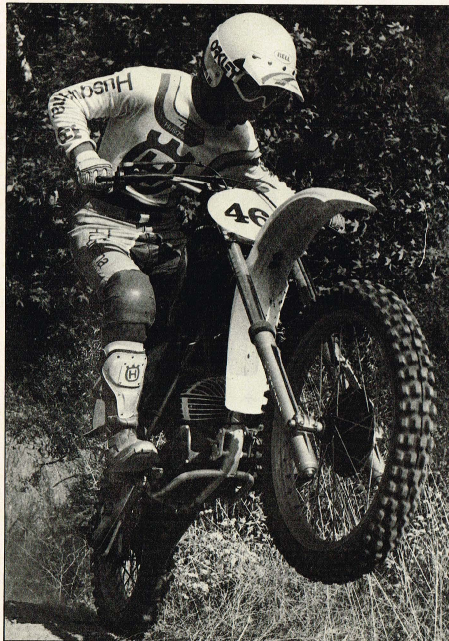
Hillclimbing usually called for first gear, and resulted in a front wheel-high attitude. Lower gearing would help.
