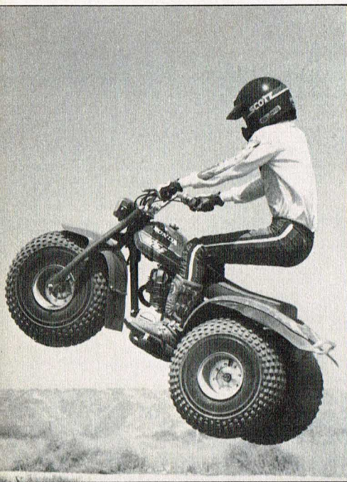
Jumping the ATC is a little risky with no suspension to cushion the landing.
