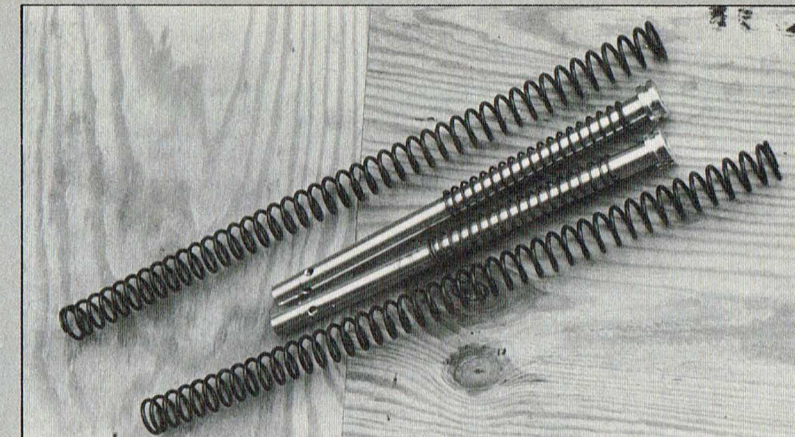
The kit comes with the rods and the fork springs. Notice the long negative springs on the damper rods. These are needed because the Simons kit requires the use of air. The negative spring keeps the ride sensitive on the smaller bumps, where air alone would be harsh.
