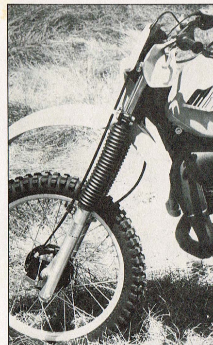
Typically fine forks on the Yamaha only required an increase of the oil level to get them working to our satisfaction. The front brake is one of the strongest around—use caution at first. Notice the tank stickers; they did this before we ever rode the bike.
