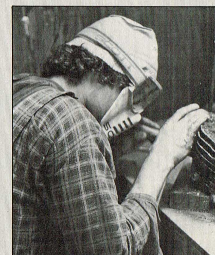
A port match-and-clean job is an effective way of adding power. Don't go nuts, the result could be an ultra fast machine that is a time bomb.
