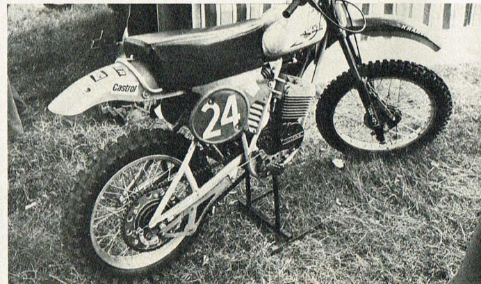
The West German Kramer, before and after. Engine is Rotax, forks are Ceriani, Boge gas shocks with remote reservoirs.
