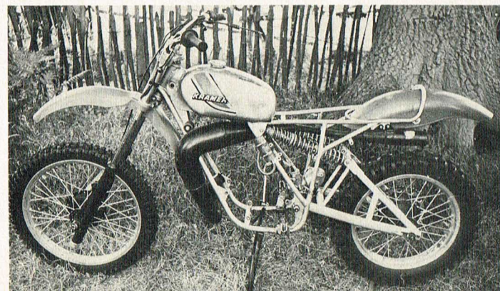
The West German Kramer, before and after. Engine is Rotax, forks are Ceriani, Boge gas shocks with remote reservoirs.
