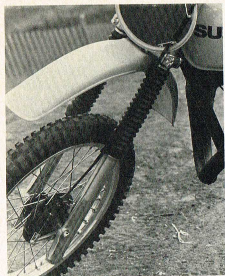
Front end travel is now up to 248mm. Although these appear to be identical to the 125 forks, they differ internally.
