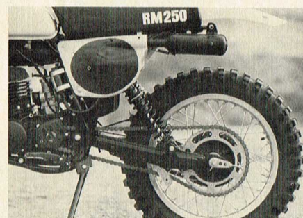
Rear end is identical to the B-model with the exception of the longer, quieter silencer that comes complete with a new mounting arrangement, and . . .
