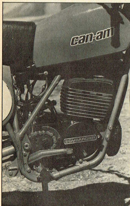
Case saver in front of the chain is to protect the ignition cover — some folks remove it to save the cases. Pegs gave a lot of support, brake pedal is super-strong.
