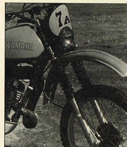
Fork travel is increased moderately to match longer rear end. Damping is good. Plastic-covered headlight, still standard, is quite durable.
