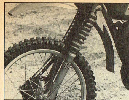
Forks are 35mm Marzocchi, orange flavor. They gave us a little over nine inches of travel, and performed flawlessly.
