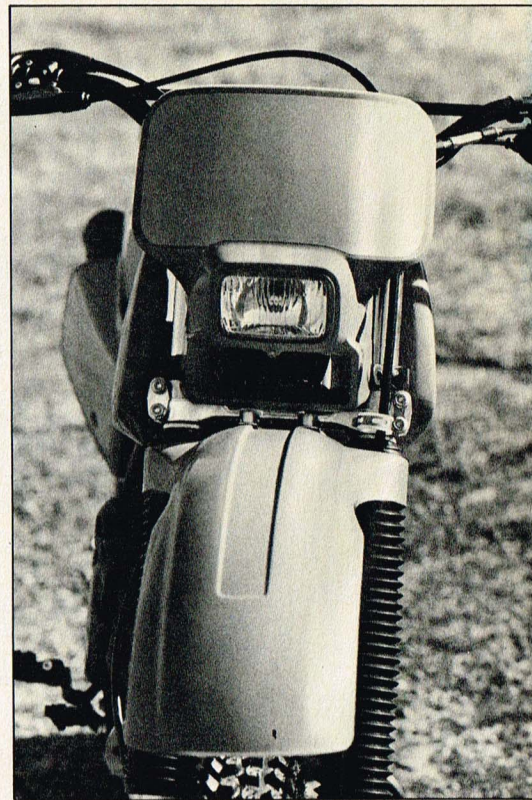
There's an optional quartz light for night riders. The front fender was designed in a wind tunnel, which is why it's flared around the forks. Supposedly, it forces air down to the motor.
