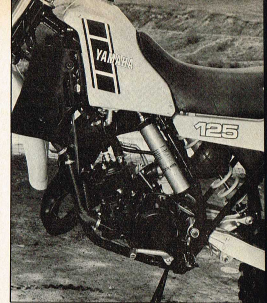
The YZ125K engine is still chockablock with plumbing and doodads, but every spare ounce of metal has been shaved away. Result? A weight of 193 pounds with an empty tank.
