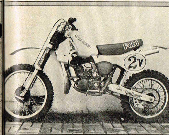
Here's the DB version of what the RM250D ought to be. Simons UDX forks up front and last year's power.
