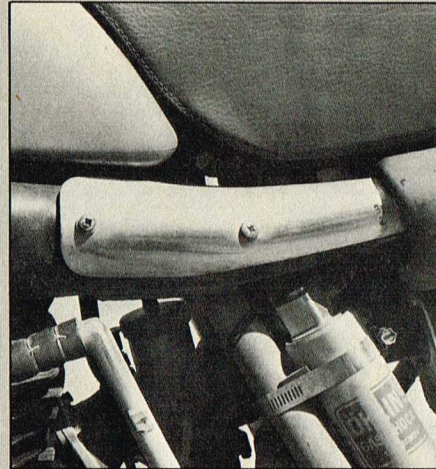
We liked the Ohlins shock the best. It was a tad more supple than the White Power shock. A heat shield is a must on the 480 pipe. We made this one out of thin aluminum.
