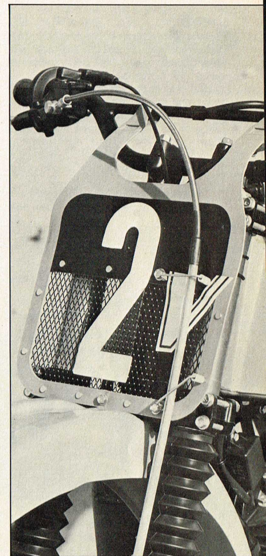
Front numberplate is wire screen and will not accept regular numbers. It's supposed to let some cooling air down to the top of the engine. Cable routing for the brake line is excellent.
