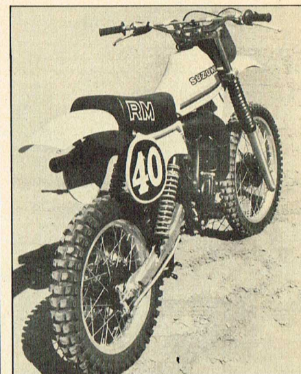
The T appears slimmer and trimmer than the N, with a higher profile rear knobby and new, longer fenders that don't snap off.
