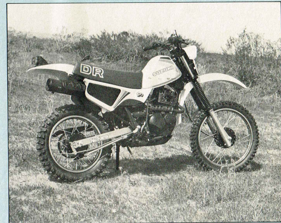
With a low seat height and a sweet chugging motor, the DR100 is a favorite among the DB staff. The suspension is advanced, even for a little bike. Floater rear, leading axle front boingers.
