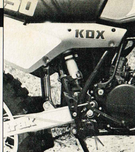
The single rear Trak link saves weight and simplifies rear-end maintenance.
