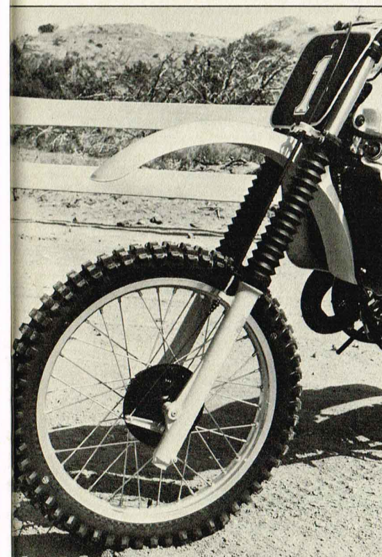
Too short forks that are harsh, plus a seriously stupid front brake cable gave bad marks to the RM.
