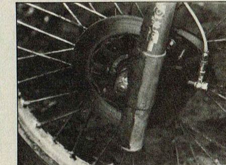
Suzuki teamsters in all classes have been experimenting with an ultra-light front disc brake. This particular assembly has been seen on the 125s and the works 250s.
