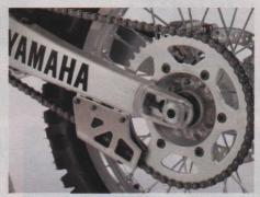
A new swingarm graces the machine, as does a lighter, stronger chain guide. The stock gearing is quite good; the stock chain is a ten-ride tear off.
