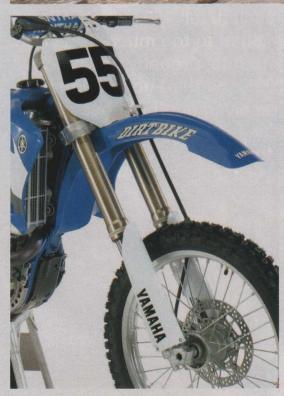
The new 48mm KYB fork is Showa-like in that it separates the oil and air. The new TCV valve is the key and makes for a better action in the fork. It's not as plush as the Showa, but craves jump faces and nasty landings.
