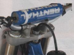
A Renthal bar is not only lighter, but stronger too. Good half waffle grips and an adjustable clutch perch highlight the cockpit.
