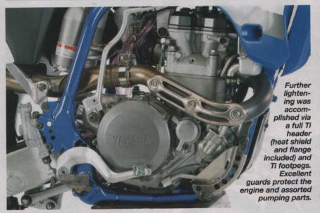
to minimize the monkey motion in the head. Remember, less reciprocating mass equals faster revs. A new 39mm Keihin FCR carburetor features a throttle position sensor and the leak jet, which is said to deliver more precise fuel/air mixture ratios. They've shaved some weight out of the motor by shrinking the cam tensioner, going to a
