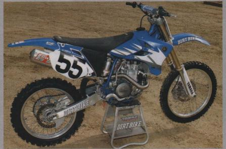
The Doctor D exhaust system not only lengthened the powerband, it sparked up the middle. Overall it made the 450 easier to ride. A taller SDG saddle is necessary for the long-legged crowd; it comes complete and is a stellar ergonomic mod.
