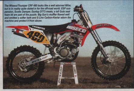
Gearing was left in standard trim (13/50) though the standard chain and rear sprocket were shelved in favor of an RK O-ring chain and Moose Racing rear sprocket.
