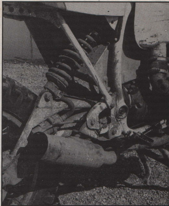
Single Bilstein damper controls the twin tube swinging arm. Under the severe stresses of the race, the damper rods gave up and frequent replacements were necessary.
