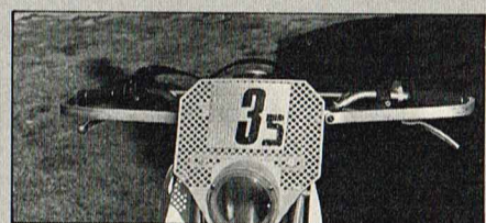
Bash bars are available from a few manufacturers, and they all perform the same function—keeping bones unbroken.
