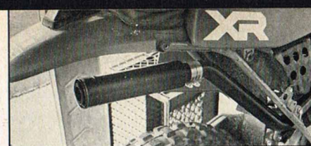
Pro-Tec headpipe with J&R muffler/spark arrester.
