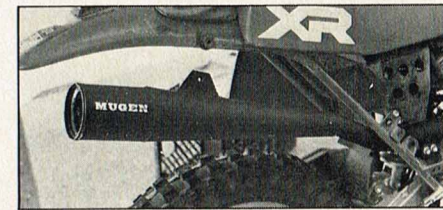
Baja proven, the Mugen steel muffler worked well.
