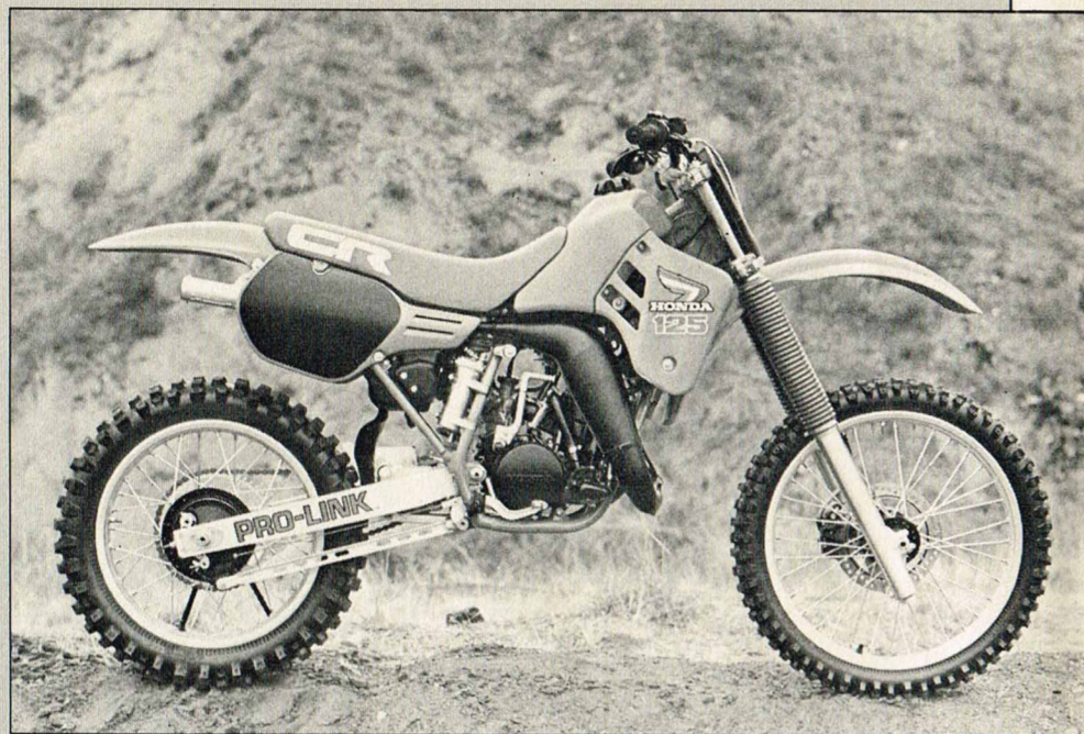
The new flat-slide Keihin carb is one of many changes on the 125 engine. They've coaxed a few more ponies out of the 125 with pipe, porting, and other minor items.
