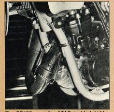
The CR125 uses the ATAC molded right into a header pipe section. Linkage is internal, driven from crank.
