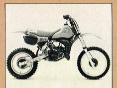
The CR80 picks up a few of the big-bike features this year, including the bolt-on rear frame section and larger-diameter forks (up to 33mm from 31mm). The engine has been completely redesigned, including the addition of a mini ATAC system, and is said to have better power delivery throughout the range. Suspension travel is up, with 9.4 inches in the front and 10.0 in the rear.
