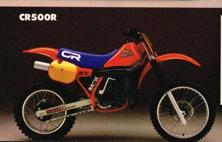
491 cc single-cylinder reed-valve Engine inducted two-stroke
