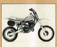
A lighter engine is one of the main features of the CR60. Part of this weight loss can be attributed to a thinner cylinder liner—designed to transfer heat more efficiently than the old, thicker liner. The 30mm forks are new, with 8.0 inches of travel; the Pro-Link rear delivers 8.3 inches. The weight remains the same as the '83 bike.
