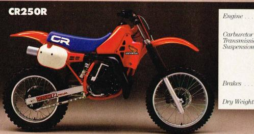
Engine 246 cc single-cylinder reed-valve inducted liquid-cooled two-stroke
