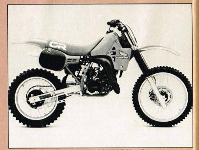
A totally redesigned engine is the main highlight on the new 125. The thrust of the new design is to increase power and lower weight. There is a slight weight gain overall due to the new 43mm forks, but fork flex should now be a thing of the past. Travel is shorter than on the big bikes, at 11.4 inches, while the rear stroke is 12.2 inches. New plastic looks sturdier, with a cleaner design.
