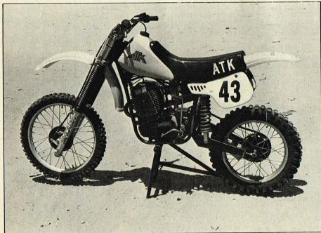
The ATK proto bike is based on a 560 Rotax engine in a special C&J frame. A version of this bike will likely be for sale in the near future. The price tag? Somewhere below the \$4000 range.
