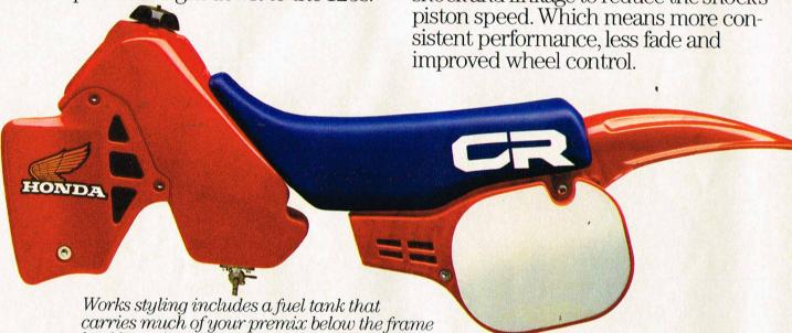
backbone for a lower center of gravity and better handling. Redesigned lightweight frame features bolt-on rear section for simplified maintenance.
