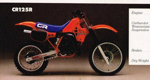
Engine 123 cc single-cylinder reed-valve inducted liquid-cooled two-stroke
