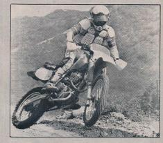
Less bulk and stiffer suspension make the new XR600R a better-handling, less-tiring package. A nikasil cylinder and other weight-saving details give the thumper a lower center of gravity, which translates into more flickability. The firmer boingers soak up big hits better, and they also feel smoother over small bumps.
