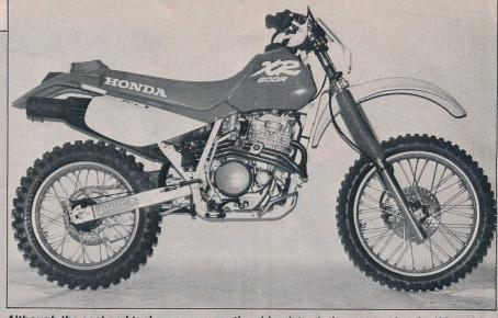
Although the seat and tank are narrower, the side plates bulge out to give the '88 a wider midsection than the '87 XR600R. Also, we had a rear-wheel bearing go out on our '87, so with the '88 using two bearings instead of three in the rear hub, longevity is in question. The tank decals die within a month. Still, the '88 is light-years ahead of last year's offering.
