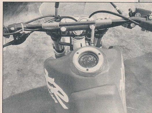
Lightning pits: A road race dry-brake quick-fill system replaces the stock cap on Ogilvie's B2V-winning XR630R. Bruce removes his headlight to allow more cooling air to the frame.
