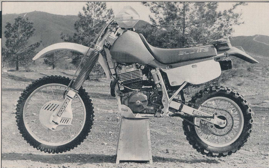
Besides CR triple clamps and a 17" rear wheel, Scott depends on a UNIK steering damper to slow things down a bit at race speeds. It's adjustable while riding.
