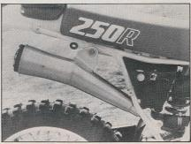
White Bros. megalloy silencer kit, with the SuperTrapp spark arrester is the only hardware mod that was made on the XR for Part One of our XR hop-up. Big weight savings are attained, and top-end power has been slightly increased with the bolt-on kit. Part Two of our story will extract the big ponies from the Honda mill.
