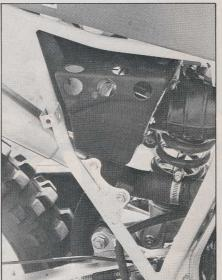
Dan White's airbox tricks include drilling five holes in the top of the airbox, and the addition of the K&N filter. When done in conjunction with adding the silencer kit, the results were a full two-horsepower increase over stock.
