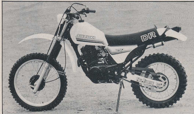
The 125 swingarm is steel, but painted aluminum. Floater rear end is decent, but not as elaborate as the 250 setup.
