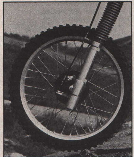
Gigantic (for a 125) 43mm KYB forks rate right up at the top in action. Even though they don't have the trick chromed finish of the 250, they are plush.
