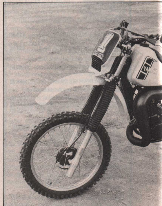
Forks are massive 43mm units. Front brake is same double-leading shoe item of the YZ465/490.
