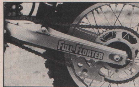
Spiffy aluminum swingarm appears unbreakable. Chain guide is nicely designed.
