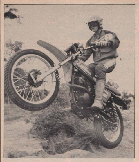
As for the handling, the SP took the roads all in stride. The trials tires on both ends left a bit to be desired in some of the climbs and fast, sliding turns, and there is really no excuse for Suzuki not putting the claw action units on this motorcycle. The suspension was very soft, but not plush. It can take the light abuse of an easy fireroad comfortably, with no hopping or skittering around.
