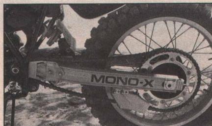
Use the new axle plates on the swingarm and the new-style chain guide does a faultless job. Loctite those two bolts on the front swingarm guard.
