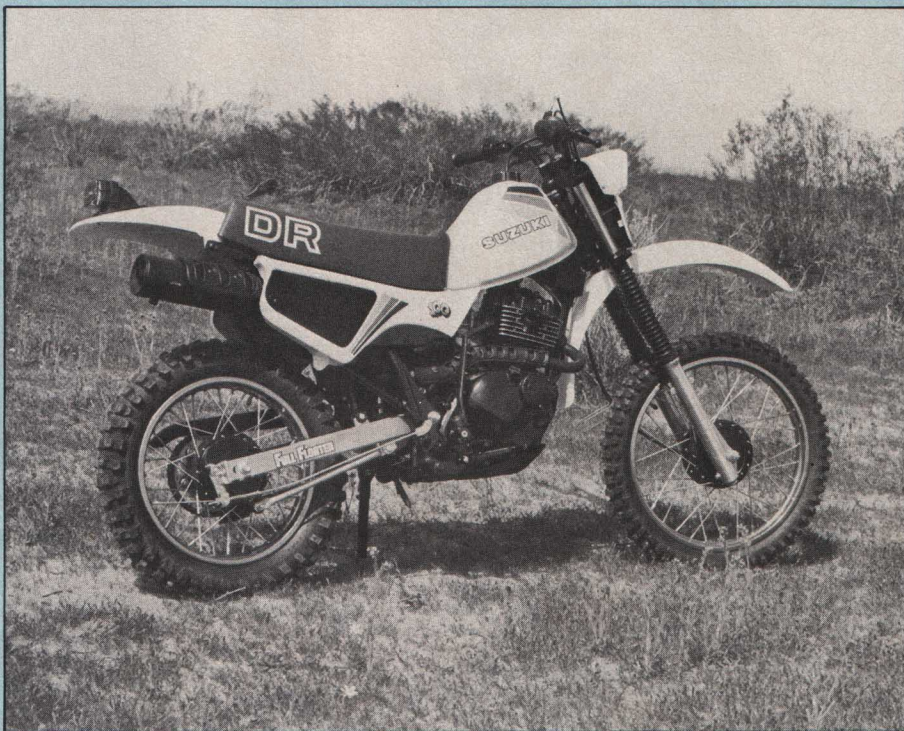
With a low seat height and a sweet chugging motor, the DR100 is a favorite among the DB staff. The suspension is advanced, even for a little bike. Floater rear, leading axle front bongers.
