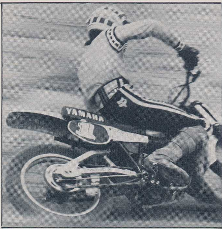
John Whelchel dives into a turn on the first of the new water pumpers. The new 27½-degree steering head angle made this a more precise maneuver.
