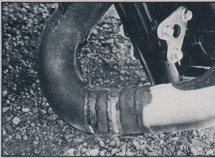
By adding 20mm to the header pipe, low-end and mid-range performances are greatly improved.
