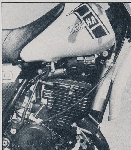
The seat/tank junction is deluxe. It allows the rider to slide forward easily. YEIS induction is new, as is the larger 490 motor.
