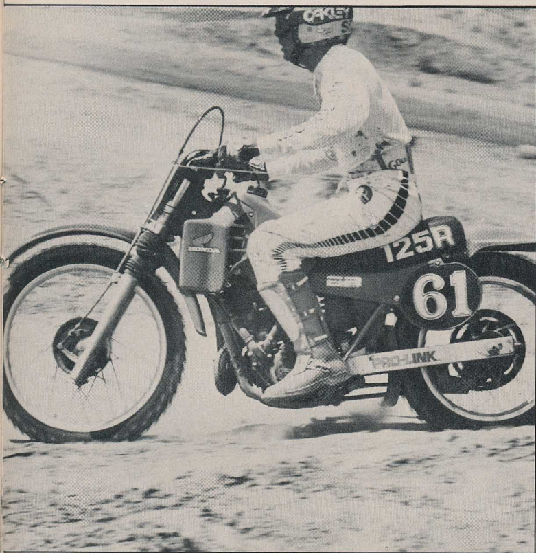
The Honda had adjustable compression damping both front and back. The Pro-Link featured a fairly high rate of progression which allowed for soft action over small bumps and firmed up over the crunchers. Shock fade was noticeable in long motos.
