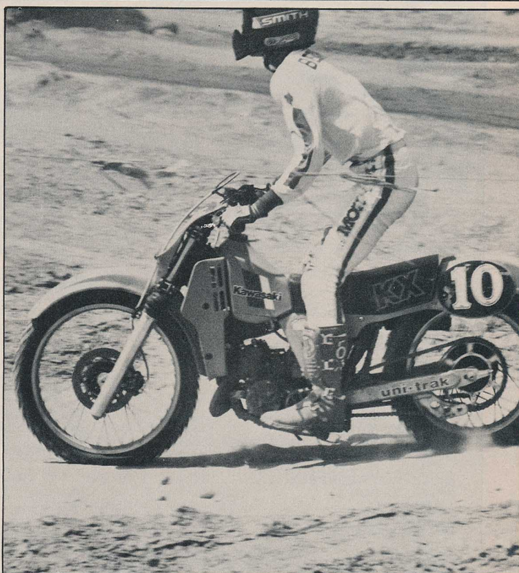
Kawasaki relocated the rocker arm and struts on the Uni-Trac to provide a rising-rate rear suspension for '82. This was a definite improvement, as the KX seemed to be one of the most stable bikes over high-speed sand whoops.
