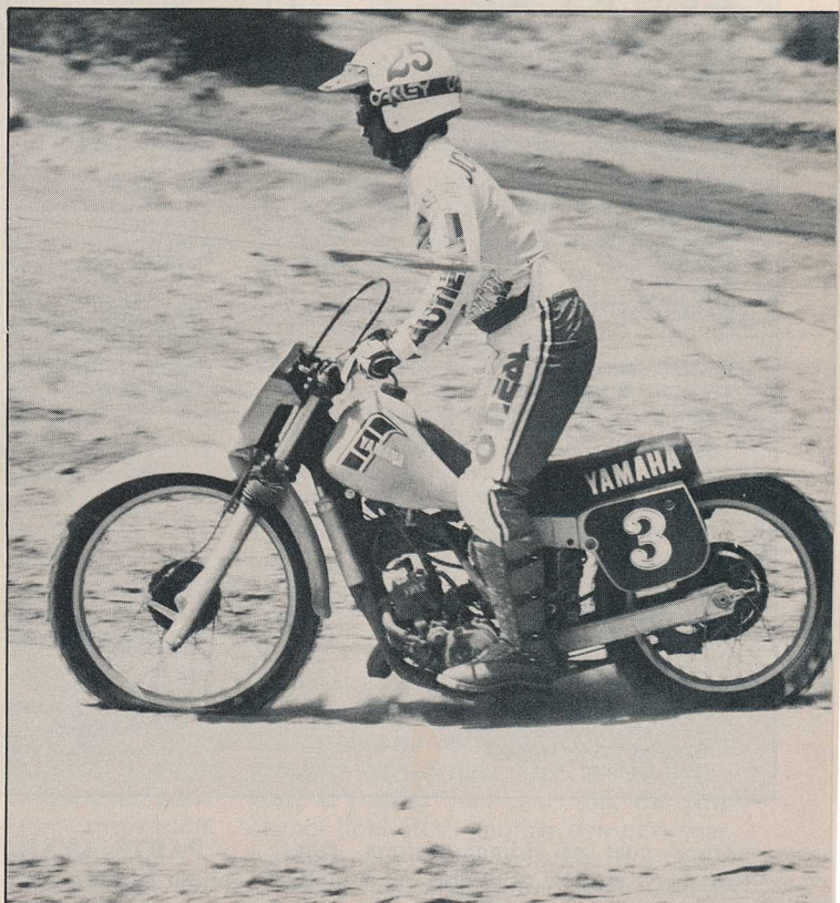
The Yamaha proved to have the best forks. At the rear it's a different story, though. The rate of rise in the Mono-X was very moderate, causing the YZ to be fitted with a spring that was adequate for small bumps, but too soft for hard landings. Bottoming out, like this, was common.
