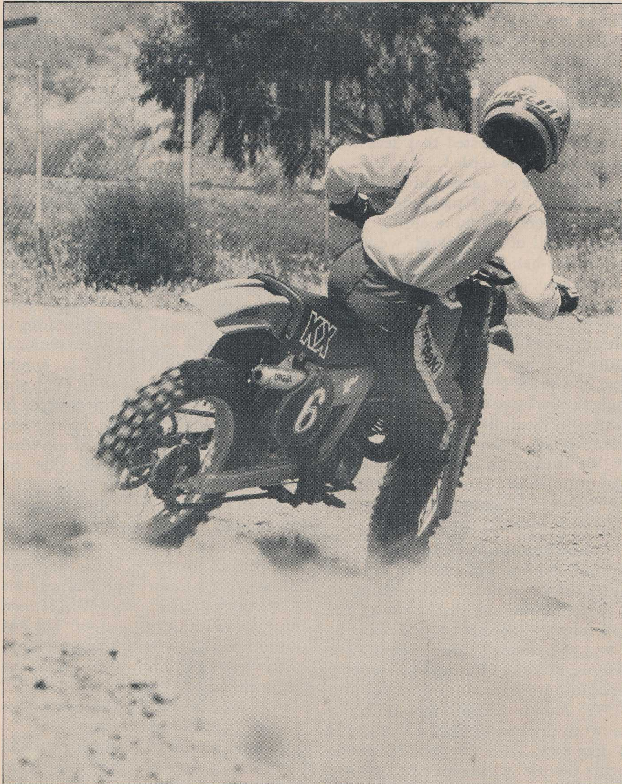
Longish swingarm lent a great deal of stability to the KX. Sliding was easy as long as the power lasted.
