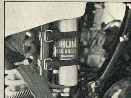
The installation of an Ohlins shock gave our Suzuki a world-class rear suspension and ended fiddling with preload.
