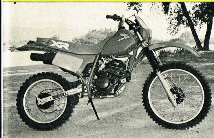
While most felt that the safety seat looks good, the big tongue limits rider mobility, making it tough to get forward in the turns.
