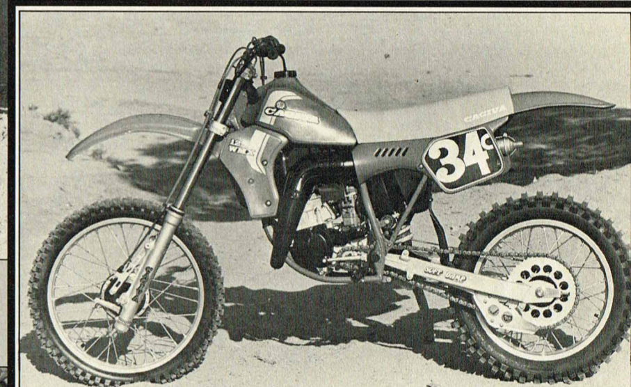
Although the shifting is smooth as pancake batter, the countershaft sprocket is placed too far from the swingarm pivot point. The rear frame section unbolts and there's a nifty heat shield on the belly of the pipe.
