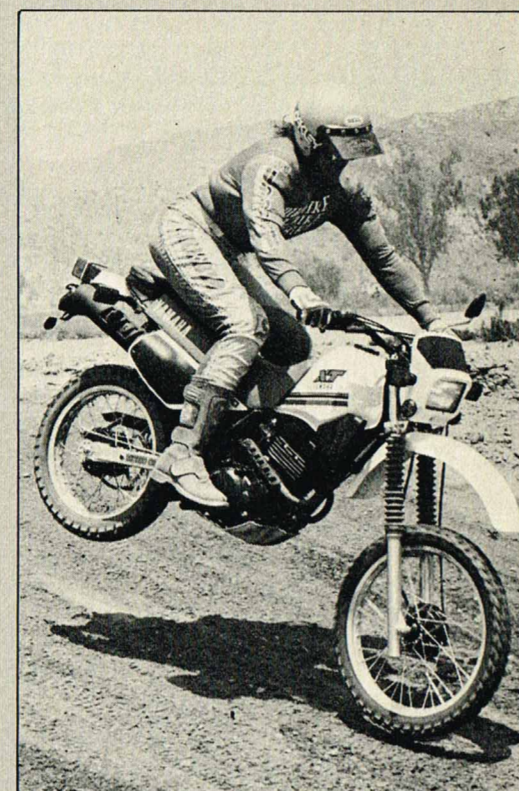
Soft suspension is fine for medium trail work, but expect some serious clanking when you jump the XT.
