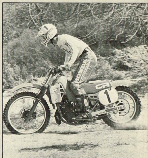
On David Bailey's practice scoot the engine is left stock and a set of works forks are installed. Both suspension ends are painfully average on the production CRs.
