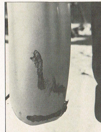
The front fender on our test bike was mounted back a little too far, and rubbed on the exhaust pipe.
