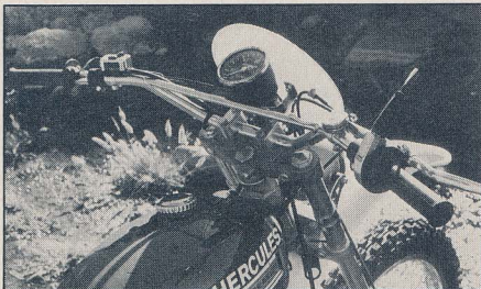
The VDO speedo and the Magura levers, throttle and grips are indicative of the first-class components the Herc sports.
