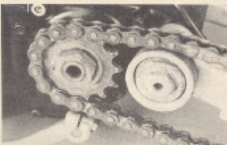
No tensioners clutter the YZ's final drive, because the countershaft and swing-arm centers are nearby.
